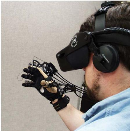
The CyberGrasp and VEST were integrated into the IST Virtual Environment Software Sandbox (VESS) and Virtual Reality (VR) testbed. These devices give participants in an immersive virtual simulation the capability to interact with the
