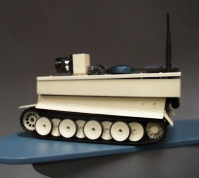
A robot with a wireless video camera and a wireless hub for transmitting real-time video to a control station.
