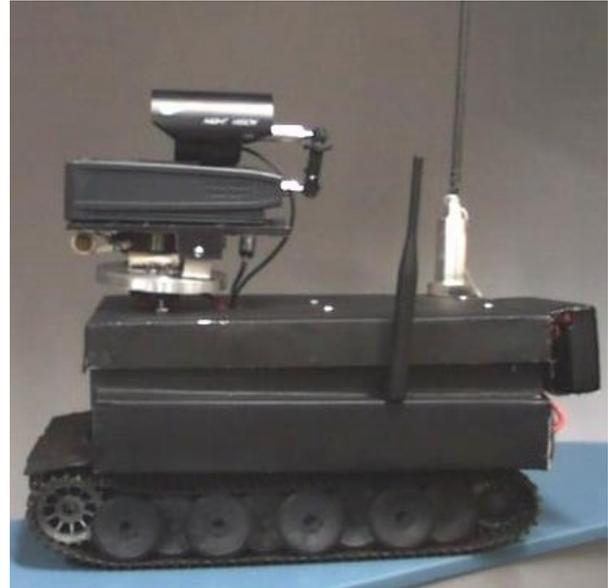
A robot with laser range finder, infrared video camera mounted. It also has a 802.11b wireless hub, Motorola GPS and JStik inside the body of the tank.
