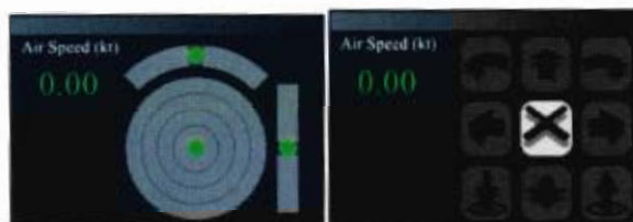
Figure 1: Two input schemes for manual control of the simulated MAV. The analog scheme (left) controls lateral movement via the center circle, altitude via the bar on the right, and rotation by the arc at the top. The digital scheme (right) uses the different buttons to control the MAV.
