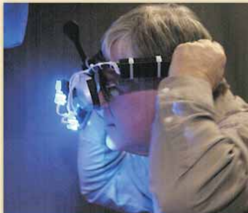
Charles Hughes checks the view using a headset with video camera eyes. The blue light bounces off retroreflective curtains directly back to the cameras. The computer substitutes digital images for the blue, providing the wearer a mixed reality view of the world.
